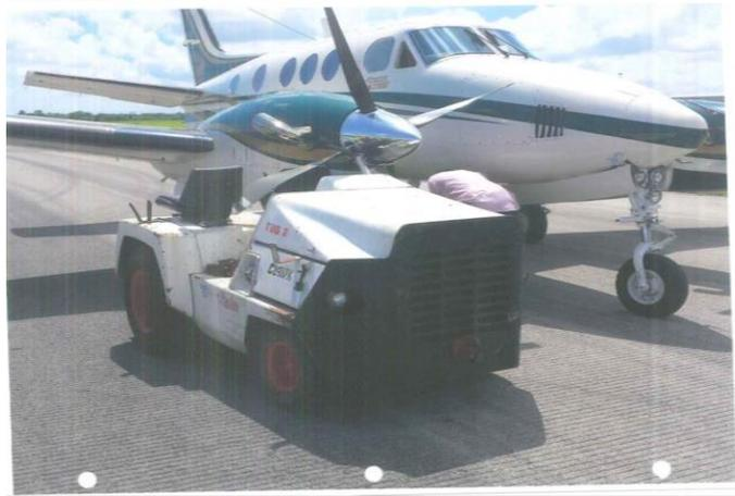
Damage to the right nacelle and propeller was really not that monetarily significant, given that it was a King Air. The owner's first decision was a question of repairing the existing parts or replacing the bent parts with new. Straightening and repairing the existing sheet metal would take 155 days. Waiting time for new replacement parts from Beech was 462 days. Since the policy didn't include the use of a replacement aircraft during the repair, the owner chose the 155-day solution.
